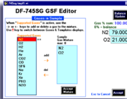
(Figure 3) - Main Screen, Supported Gases Display
